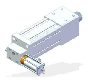
Special actuator with double motions, linear and rotating of the piston rod. Linear cylinder  $\emptyset$  80 mm., stroke 100 mm., piston rod diameter 40 mm., with increased bushing guide, rotation of the piston rod of 90° by grooved rod and bush in sintered bronze. Cylinder for actuating the rotation  $\emptyset$  25 mm., with adjustable stop.
