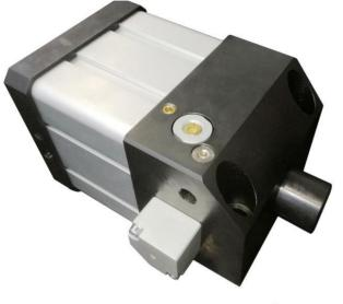
Special actuator for locking of mould integrated with cylinder Ø 125 mm., stroke 30 mm., double acting, magnetic piston, pneumatic adjustable cushion for the return stroke, front head in steel with piston rod in high resistant steel and thermal treatment for further hardening of the surface, security device for locking of the piston rod in extended position.
