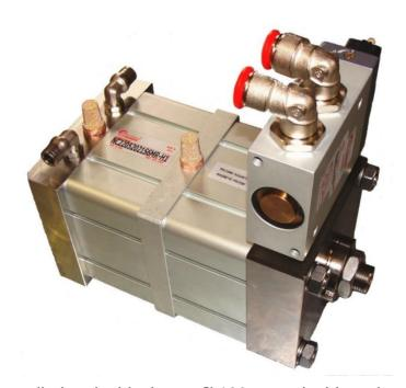
Tandem compact cylinder, double thrust, Ø 100 mm., double acting, magnetic piston, mechanical adjustment of the return stroke and with integrated control solenoid valve.
