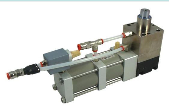
Special actuator for "mould closure" with tandem pneumatic cylinder Ø 80 mm. and cylinder Ø 63 mm., angular mechanical group for increasing the force, piston rod in high resistant steel, piston rod seals and grease certificated for food industry.
