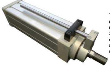
Telescopic cylinder dual steps. First stage Ø 100 mm., second stage Ø 70 mm., total stroke 550 mm., piston rod in chromium steel C45 diameter 30 mm., anti rotation system on second stage, caps in anodized aluminium, tube of the first stage in profiled aluminium, tube of the second stage in chromium steel E355.
