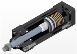
Double acting cylinder series ISO15552, Ø 50mm., stroke 75mm., caps and tube in aluminium protected by epoxy painting, piston rod and screws in stainless steel AISI 304, with integrated internal spring for security guarantee.
