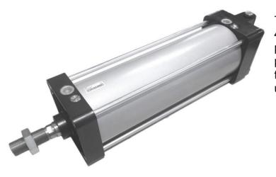
Tie-rod CNOMO cylinder, Ø 200 mm., stroke 400 mm., tube in steel internally chromium plated and epoxy painting, caps in aluminium painted, special execution with piston seal for fast sliding, guide runner in carbo-graphite, used to balance masses in fast movement.
