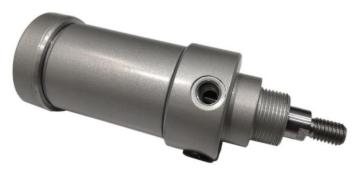
Round cylinder with screwed caps "interchangeable" with the old model of Pneumatica Italiana, Ø 40 mm., stroke 40 mm., single acting front spring, mounting by front threaded cap.
