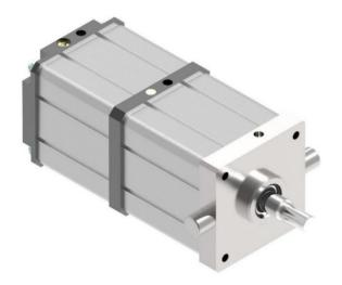
Compact cylinder, tandem in thrust, caps in melting of aluminium, front cap in steel with integrated rotation pins, rear and intermediated caps in anodized aluminium, profiled tube in anodized aluminium, increased piston rod diameter 32 mm., adjustable cushion only on return stroke.
