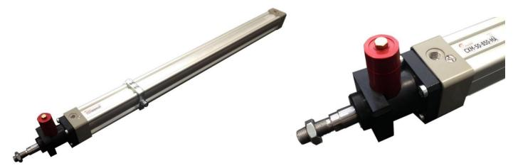
Cilinders ISO15552 Ø 32,40,50,63,80,100 mm., available for several strokes, with integrated mechanical device for locking the piston rod and intermediate adjustable hinge for oscillating fixing.
