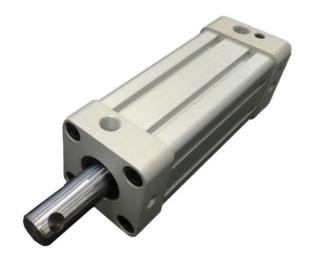
Cylinder originated from series CX according ISO standards, double acting,  $\emptyset$  50 mm., stroke 90 mm., caps in aluminium machined from solid bar, profiled tube in anodized aluminium, piston rod diameter 20 mm. in chromium plated steel, piston and piston rod seals in PTFE loaded and energized by spring, guide band on the piston in bronze, suitable for functioning up to 300°C.
