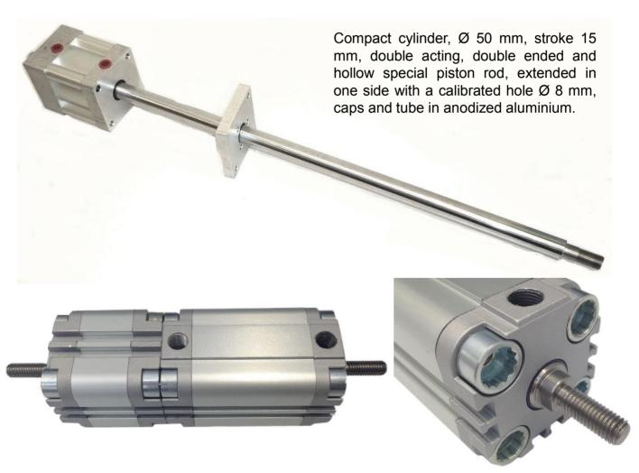
Compact cylinder series CU  $\varnothing$  32mm., version opposed tandem cylinders with piston rods  $\varnothing$  16mm. with internal precise antirotation piston rod device.
