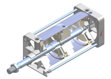
Cylinders series ISO15552 Ø 160 and 200 mm., tandem version with double thrust, tie-rod construction, with caps and tube in aluminium protected by epoxy painting, piston rod and tie-rods in stainless steel AISI 304.
