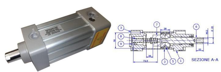
Tie-rod cylinder series ISO15552, working with compressed air up to 16 bars and high vacuum, single acting, without air the piston rod is out with springs integrated in the rear chamber, used for security functions in autoclaves with high vacuum.
