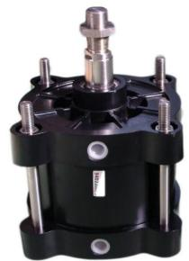
Tie-rod compact cylinder, Ø 250mm, stroke 75 mm, without adjustable cushions, with steel tube internally hard chromium plated and externally epoxy painted, caps in die cast aluminium epoxy painted, piston rod and tie-rods in stainless steel AISI 304.
