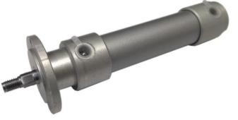
Round cylinder with screwed caps "interchangeable" with the old CP model of Bonesi Ettore, Ø 27 mm., stroke 80 mm., double acting, mounting by front flange.
