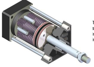
Tie-rod cylinder,  $\varnothing$  125 mm., stroke 55 mm., single acting with piston rod out without air and integrated springs in the rear chamber, piston rod in stainless steel AISI 303 and piston seal in Viton.
