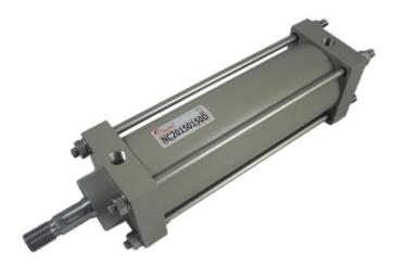
Tie-rod cylinder, Ø 63 mm., stroke 150 mm., tube in steel internally hard chromium plated and epoxy painting, special execution with piston seal for very high speed sliding, guide runner in carbo-graphite and special grease for high performances, for functioning in "positioning" linear actuators.
