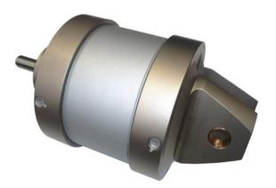
Round cylinder with screwed caps,  $\emptyset$  220 mm. stroke 100 mm., caps in chemical nickel plated aluminium, rear cap with integrated hinge, tube in nickel plated brass with epoxy painting, piston rod in stainless steel AISI 304.
