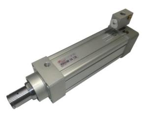
Cylinder originated from the series CX according to ISO15552 standards, Ø 63 mm. stroke 125 mm., double acting, piston rod diameter 40 mm. in C45 chromium plated steel with terminal according customer design, profiled tube anodized aluminium, integrated lock valve one way pneumatic actuated with ports G1/4".
