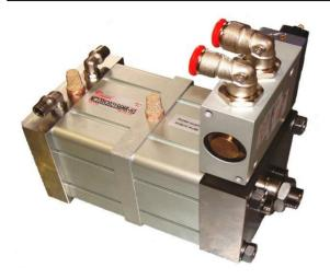
Tandem compact cylinder, double thrust,  $\emptyset$  100 mm. stroke 25 mm., double acting, magnetic piston, mechanical adjustment of the return stroke and with integrated control solenoid valve.
