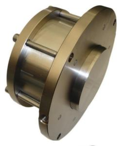
Special compact cylinder for thermo sealing machines, food packaging field, piston Ø 180mm. stroke 25 mm., double acting, front and rear caps in anticorodal aluminium chemical nickel plated, piston and piston rod in stainless steel AISI 304, tube in stainless steel AISI 304, FKM (Viton) seals for high temperature.
