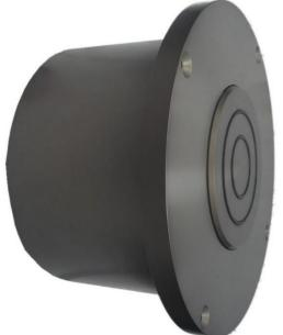
Special compact cylinder for thermo sealing machines, food packaging field, piston  $\varnothing$  180 mm. stroke 30mm., double acting, front cap and barrel in anticorodal aluminium with hard anodization, piston and piston rod in aluminium with hard anodization, FKM (Viton) seals for high temperature.
