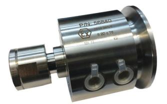
Round cylinder Ø 50 mm. stroke 10 mm. double acting with safety spring, 2" front flange mounting "clamp", made completely in stainless steel A316L with fine end stroke adjustment system, laser print of technical data and customer logo, ATEX certification.
