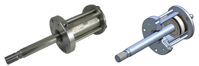
Round tie-rod cilinder Ø 80 mm., stroke 50 mm., caps and tube in stainless steel AISI 304, extended piston rod in AISI3 04, seals in FKM (Viton).
