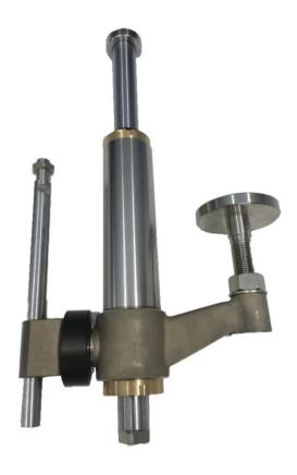
Cilynder Ø 100 mm. stroke 70 mm., single acting, piston rod, piston, caps in stainless steel AISI304; rounded tube in hard chromium plated steel, epoxy painted, piston seals in energized P.T.F.E., guide ringe in P.T.F.E.
