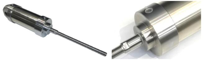
Round profile cylinder Ø 85 mm., stroke 140 mm., caps in steel AISI 304 connected by screw to the tube in nickel plated brass, rear cap with integrated hinge, piston rod in AISI 316 steel with extended thread.
