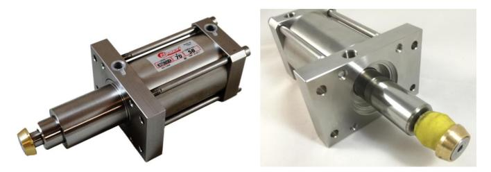
Cylinder Ø 70 mm., stroke 58 mm., totally in stainless steel AISI 304, tie-rods construction, double acting with pressure up to 16 bar, double ended piston rod with internal through hole for the passage of the air, double movement of the piston rod by compression of the front seal.
